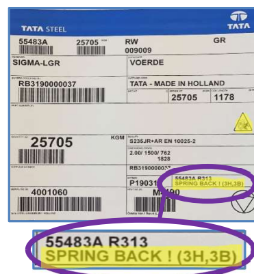
Figure 2 Customer label with spring back indication and the minimum number of circumferential and bore bands on the naked coil. This coil requires 3 circumferential bands (3B) and 3 bore bands (3H). For cold wound material only the minimum number of circumferential bands is indicated.
