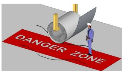
Figure 3 banding should never be removed from a coil suspended from an overhead crane or forklift.
